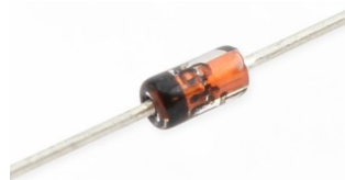
1N4148 diode (3mm long) Typical Si signal diode.
